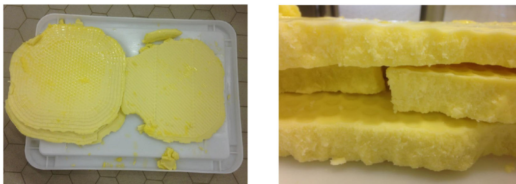
FIGURE 4 Top view and side view of filter cakes produced in the pilot plant filter press. The membrane side is up. The thickness of the cakes is almost 25 mm [Color figure can be viewed at wileyonlinelibrary.com ]
