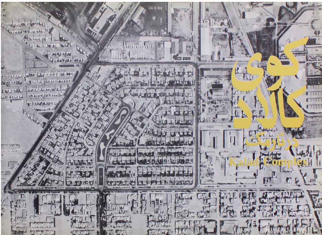
Figure 3. A sub-neighbourhood of Narmak constructed out of 310 houses with KALAD system. Source: Iran Housing Organisation Report (Tehran: Offset Press, 1972), 126.
