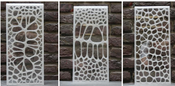
Figure 3. Glass panels (3D-printed PETG Voronoi core) (Neeskens, 2018)
