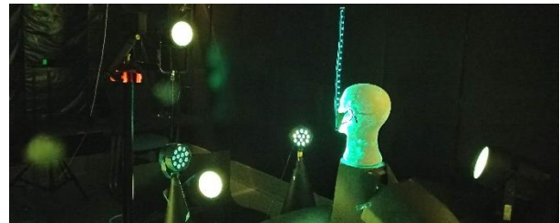
Figure 1: Setup in the Experience Room with Styrofoam head, UV lights, and black backgrounds.
