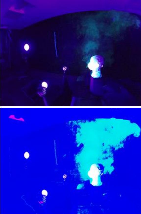
Figure 2 Same picture in 50th second, as raw footage and after background subtraction.
