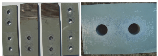
Figure 7. Specimens tightened with M20 bolts after testing
