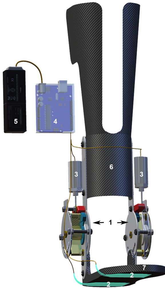
Fig. 2. ADJUST - right-leg version. 1 = lateral and medial mechanical hinge, 2 = force sensing resistors (FSRs), 3 = solenoids, 4 = cased Arduino board, 5 = battery, 6 = shank cover, 7 = footplate. The footplate is inserted into a shoe (not shown) and the FSRs are placed underneath the sole on the heel and the metatarsophalangeals. The battery powers the Arduino, the solenoids and the FSRs. Specifications of parts 2 - 7 can be found in the Appendix. ADJUST weighs 1.6kg.
