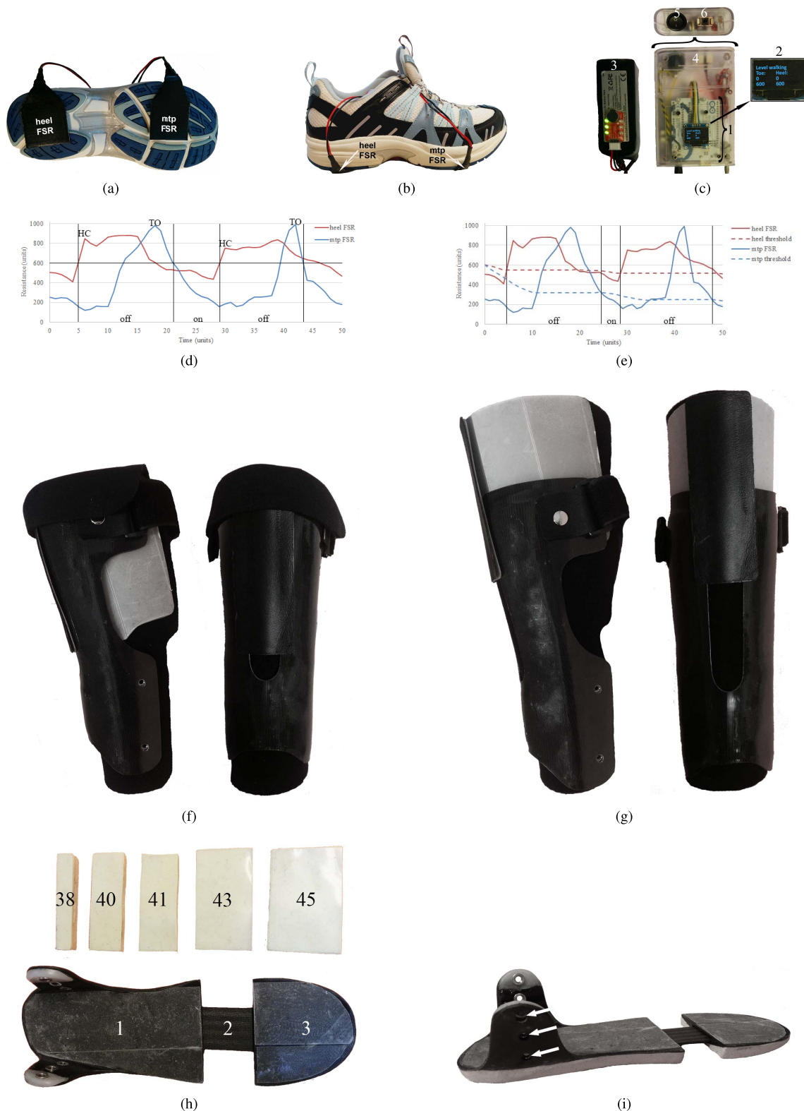
Fig. 6. Parts of ADJUST: (a,b) FSR placement; lateral (a) and caudal (b) view, (c) Arduino system, (d, e) FSR signal; fixed threshold ( \pm 44\% ON-time/GC) (d) and adapting threshold ( \pm 9\% ON-time/GC) (e), (f, g) shank cover: not extended (27cm) (f) and extended (34cm) (g), (h,i) foot plate: with spacers (h) and with height adjustments (i). FSR = force-sensing resistors, GC = gait cycle, HC = heel contact, mtp = metatarsophalangeal, TO = toe off. c) 1 = Arduino Uno R3 programming board, 2 = OLED display module, 3 = lithium polymer battery, 4 = transparent case, 5 = ON/OFF switch, 6 = push button to change program. Type of information on the OLED display (top to bottom): the program selected (walking on a level surface), FSR signal (Toe or Heel), FSR input signal (currently 0 for both FSRs), threshold for each FSR (currently 600 for both FSRs). d, e) FSR data and solenoid activation while the patient is walking on a level surface. The resistance ranges from 0 to 1,023 units. The dotted lines indicate the thresholds for the heel FSR and the mtp FSR to identify the stance and the swing phases. h) Extendable footplate with 1 = heel part, 2 = carbon plate, 3 = toe part, 38 – 45 = spacers. Foot plates without and with spacers (with corresponding stiffness in Nm/°) are available in sizes: 36 (0.23), 38 (0.27), 40 (0.42), 41 (0.42), 43 (0.50), and 45 (0.55). i) Height adjustments (arrows) make it possible to change the height of the mechanical hinges by 1.5cm.
