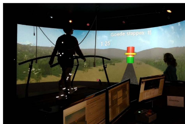
Fig. 1. Experimental set up used for the investigation. Subjects walked on the split belt treadmill while a virtual reality environment was projected onto a 180° screen in front of them. The yellow bar in the centre of the screen moved up and down with the height corresponding to the average KAM value over the first peak of the preceding step. The green region represented the target KAM, 10% reduction from baseline, and the red region represented KAM above the baseline. (For interpretation of the references to color in this figure legend, the reader is referred to the web version of this article.)
