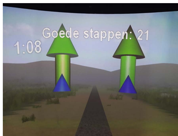
Fig. 1. Real-time feedback as seen by the patient while walking on the treadmill. The blue arrows represent the current position of the feet, with the larger arrows in the background representing the target angle. The difference between the actual and target angle is given by the colour of the large arrows (green is on target, orange is \geq 2^\circ and \leq 5^\circ either side of the target, red is > 5^\circ either side of the target). The patient aims to align their actual foot progression arrow with the target arrow of the left and right foot separately resulting in green arrows when the actual and target angles are the same. (For interpretation of the references to colour in this figure legend, the reader is referred to the web version of this article.)
