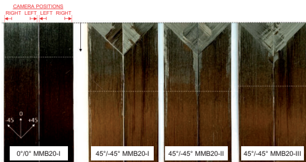
Figure 17. Fracture surfaces of MMB 20% specimens.
