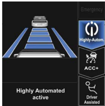
Fig. 1: A possible combination of three display components. These components were proposed in the HAVEit project as essential. From [8].
