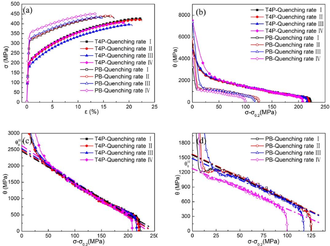
Fig. 11 – Mechanical behaviors of alloys in the different conditions, (a) true stress–strain curves for different quenching rate alloys, (b)  $\theta$  vs. ( $\sigma - \sigma_{0.2}$ ) for the alloys in (a), (c) strain hardening of alloys at T4P state, partial enlarged view from (b), (d) strain hardening of alloys at PB state, partial enlarged view from (b) (T4P + 2%pre-stretch + 185 °C/20 min).
