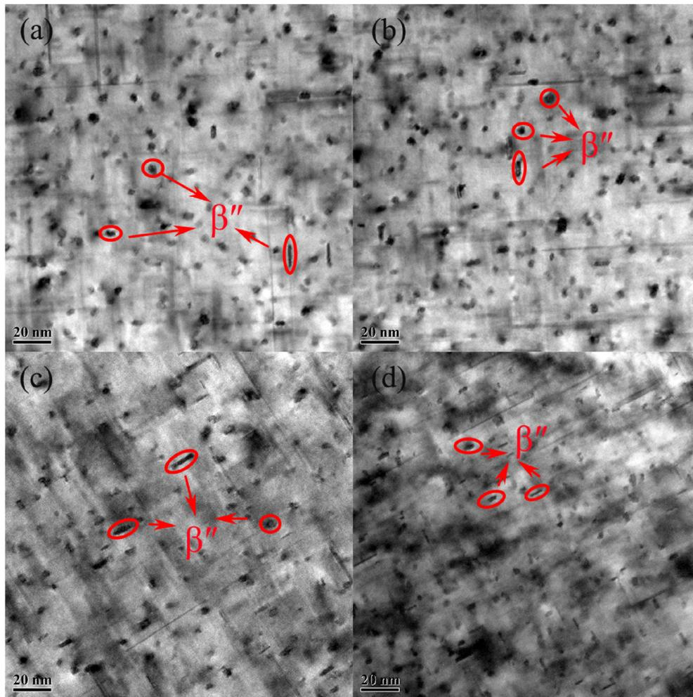
**Fig. 8 – The distribution of precipitates formed in the alloys after pre-aging + peak aging treatment of 185 °C/3 h, (a) quenching rate I, (b) quenching rate II, (c) quenching rate III, (d) quenching rate IV.**
