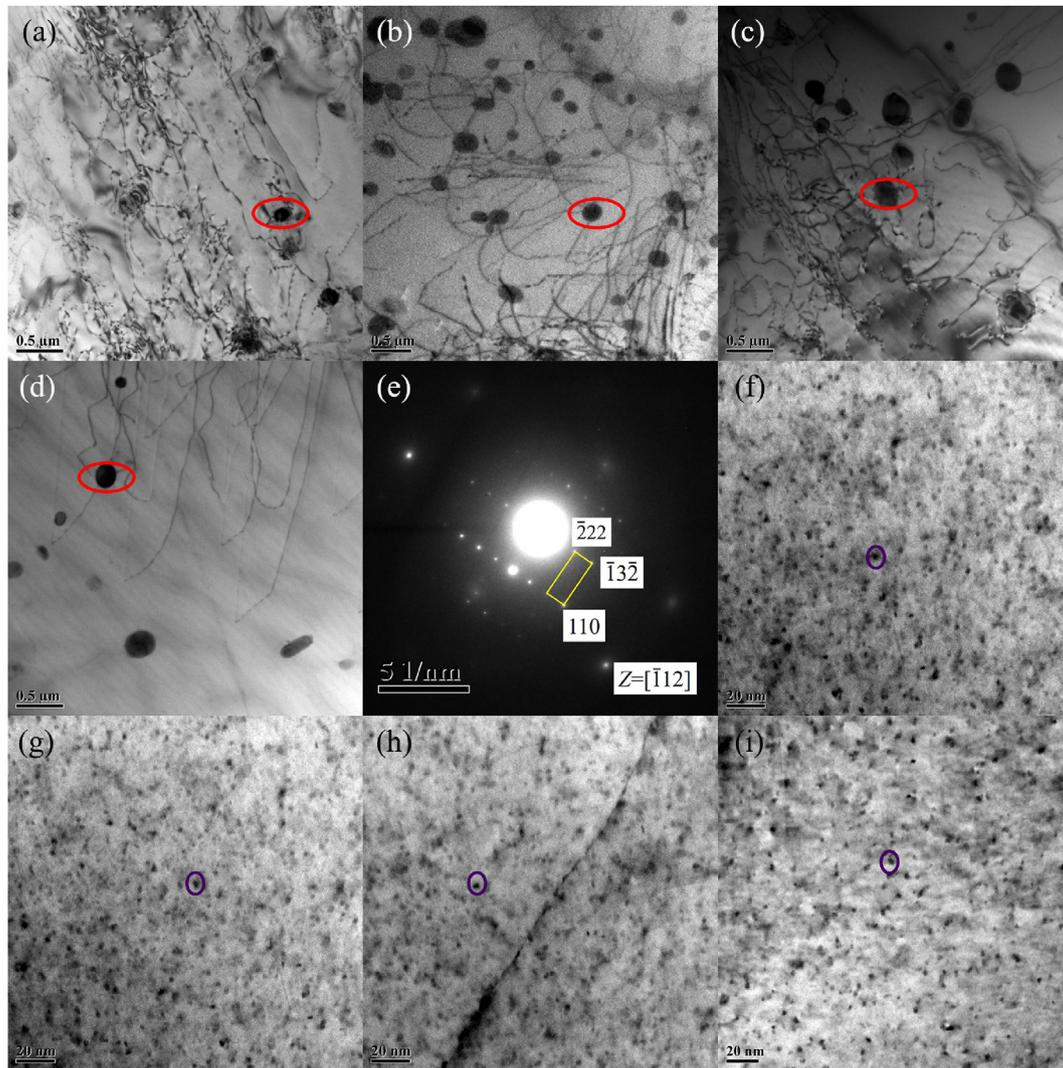
**Fig. 7 – The distribution of dislocation and second phases in the alloys after pre-aging + aging treatment of 185 °C/20 min, (a), (f) quenching rate I, (b), (g) quenching rate II, (c), (h) quenching rate III, (d), (e), (i) quenching rate IV, (e) the diffraction pattern of iron-rich phase (the phase in the red circle).**
