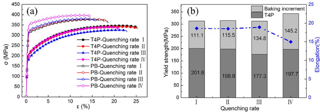
**Fig. 6** – the mechanical properties of alloys in the different aging states, (a) the engineering stress–strain curves in the T4P and PB state, (b) the YS increment and elongation after the PB treatment.
