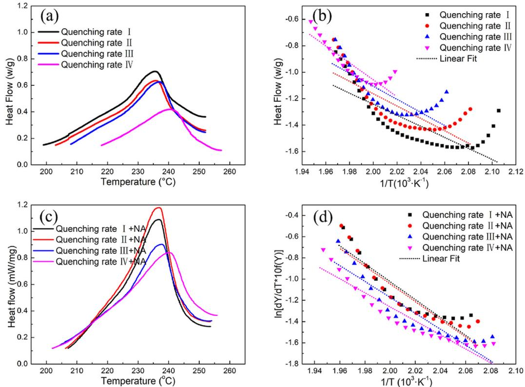
**Fig. 3** – The  $\beta''$  phase formation zones of four different kinds of quenching rate alloy in pre-aging or pre-aging + 14 day natural aging state (a), (c), corresponding activation energy diagram (b), (d).
