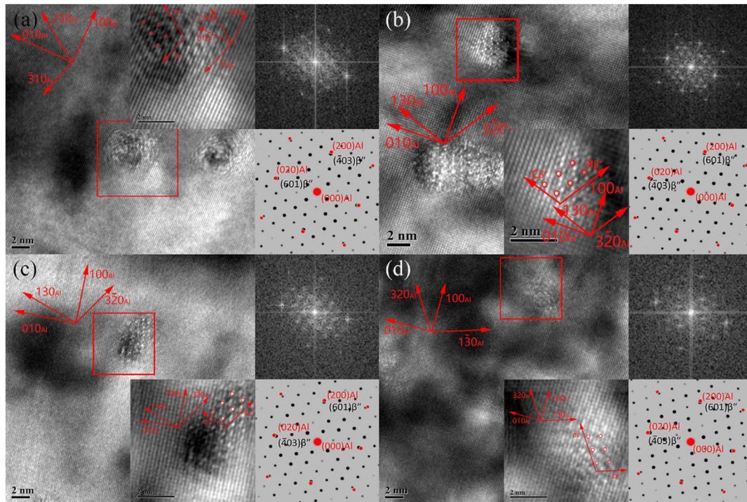
**Fig. 9 – The HRTEM characterization of  $\beta''$  phases formed in the alloys after pre-aging + peak aging treatment of 185 °C/3 h, (a) quenching rate I, (b) quenching rate II, (c) quenching rate III, (d) quenching rate IV.**
