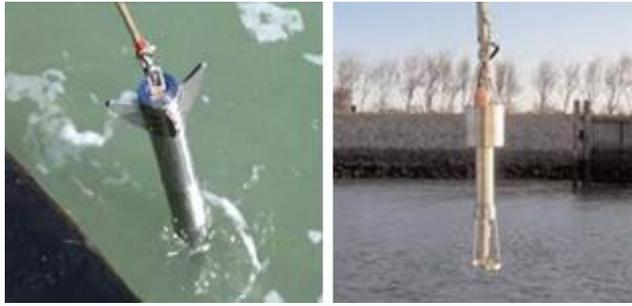
Figure 1-7 Left: the Graviprobe. Right: the Rheotune
