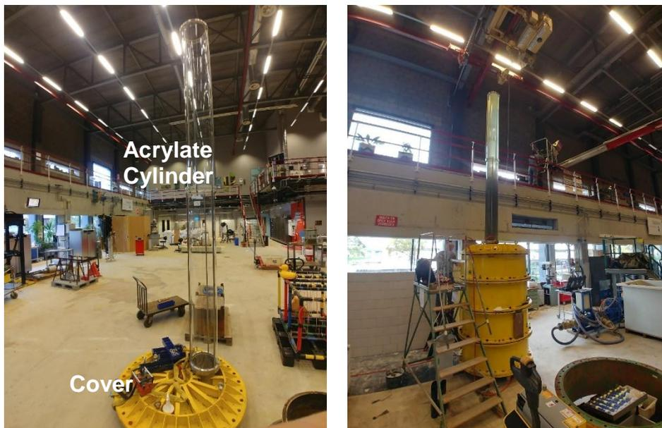
Figure 3-2: Container cover with additional acrylate cylinder.
