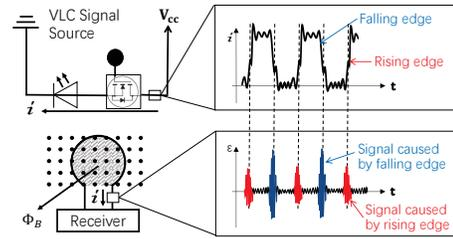
Figure 3: Illustration of the side channel of VLC.
