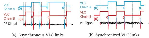
**Figure 2: Received side-channel signal from two VLC chains.**
