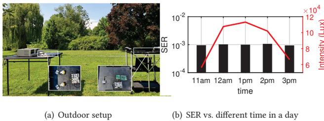
**Figure 25: Outdoor evaluation:** (a) setup; (b) SER result.
