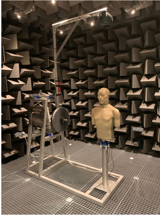
Fig. 3. The HRTF measurement system: mechanical apparatus, loudspeaker, and KEMAR mannequin.
