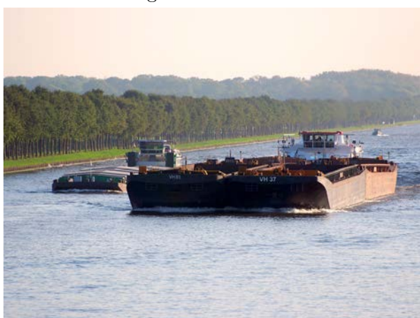
4-barge push-tow unit CEMT-class VIb
