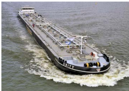
Large Rhine vessel CEMT/RWS-class Va/M8
