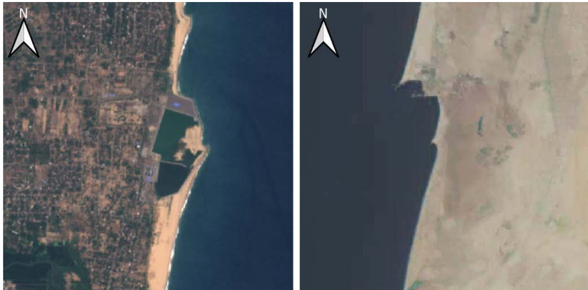
Figure 2.24: Left: Harbour siltation, Oluwil Port, Sri Lanka; right: updrift accretion, downdrift erosion, Port of Nouakchott, Mauretania. Images from Sentinel-2 cloudless by EOX IT Services GmbH are licensed under CC BY 4.0.
