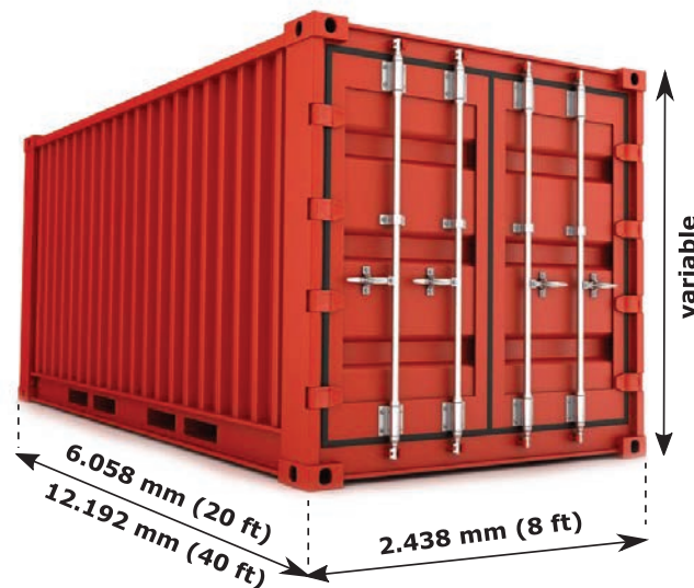
Figure 4.10: ISO container dimensions (by TU Delft – Ports and Waterways is licenced under CC BY-NC-SA 4.0).
