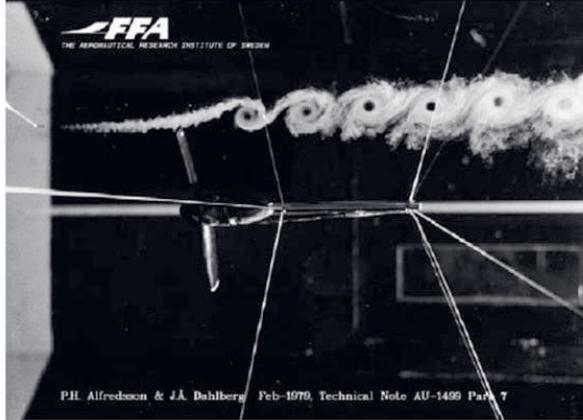
Figure 1.10: Smoke visualisation of vortices being shed at the tip of a wind turbine rotor<sup>12</sup>.
