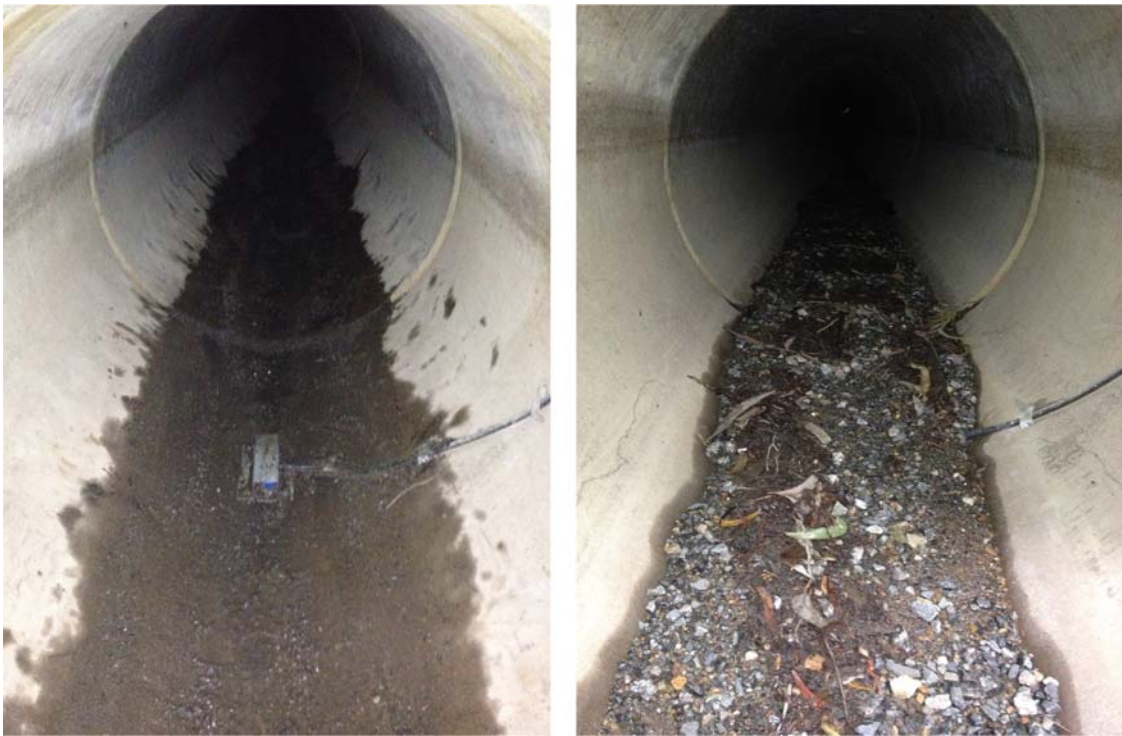
Figure 4.4 Example of a flowmeter being covered by sediments after a storm event, leading to loss of reliable data. In this case sediment accumulation was due to the construction of a small weir downslope of the probe. Source: Peter Poelsma (University of Melbourne).
