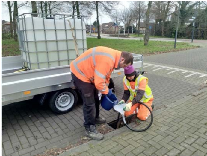
Figure 6.17 Pouring cold water onto the cable, in the underground sewer, using a hose and a funnel for validation of the measured distances by the DTS system. Source: courtesy Remy Schilperoort (Partners4UrbanWater).
