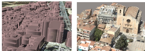
Figure 4 Current LoD1 model without textures and the LoD2 model textured using oblique images
