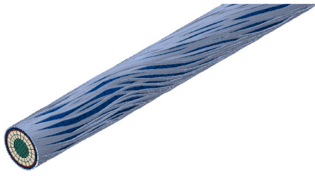
Fig. 28. The deformation of the wires in Layer V under clockwise torque with frictionless contact after slip.
