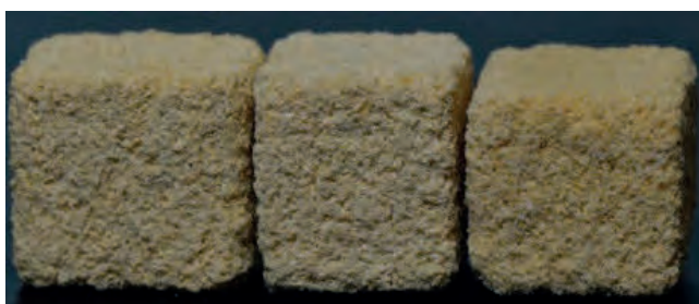
Figure 5: Untreated Maastricht limestone (left), Maastricht limestone treated with the solution of calcium citrate (middle), Maastricht limestone treated with calcium citrate and MTEOS (right).
