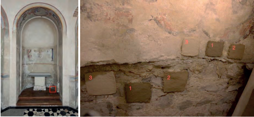
Figure 4: Specimens of 15x15x2 cm were placed on the masonry without plaster, and tests of smaller dimensions 10x10x1 cm were placed on the above mural painting in the apse.
