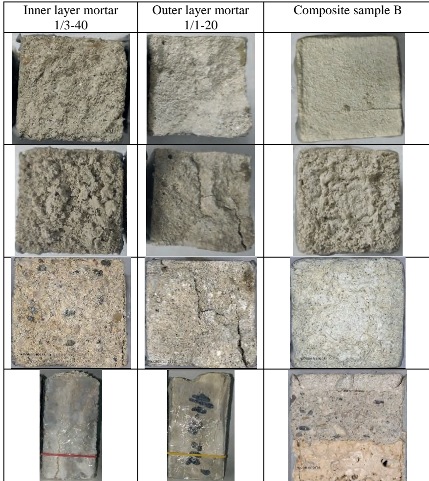
Figure 6: Composite and standardized specimens with rendering mortars 1/1-20 and 1/3-40 after 1 st , 3 rd and 5 th cycle, treated with Na 2 SO 4 solution.
