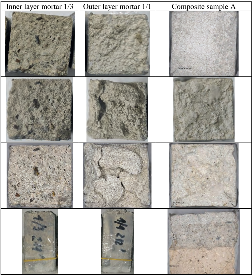
Figure 5: Composite and standardized specimens with rendering mortars 1/1 and 1/3 after 1 st , 3 rd and 5 th cycle, treated with Na 2 SO 4 solution.
